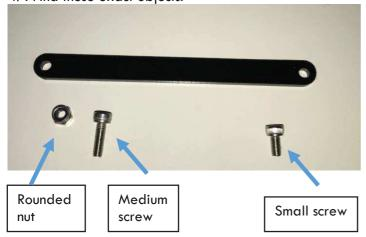
48. Use the medium screw and the nut to attach one side of the plastic piece to the piece that is connected to the Arm servo. If you need the servo to move, use the potentiometer instead of moving it with your hands.
