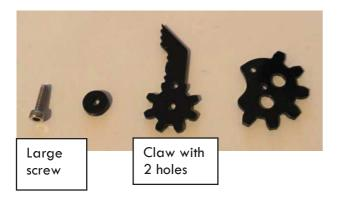
63. On the right side of your grip servo, put in the screw, then the circle, then the grip. Make the grip fit nicely with the other one grip.
