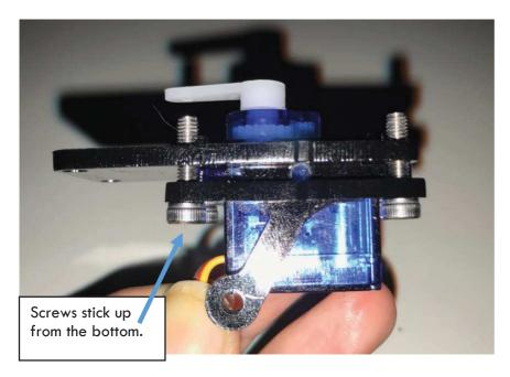
59. Take the white blade off the Grip servo. Use a pointy servo screw to connect it to this object.
