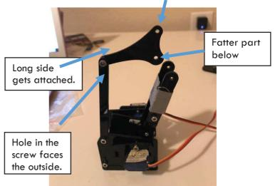
46. Find these exact objects. Flip your robotic arm around. Use the screw to attach the middle of the plastic piece to the other arm on the other side.
