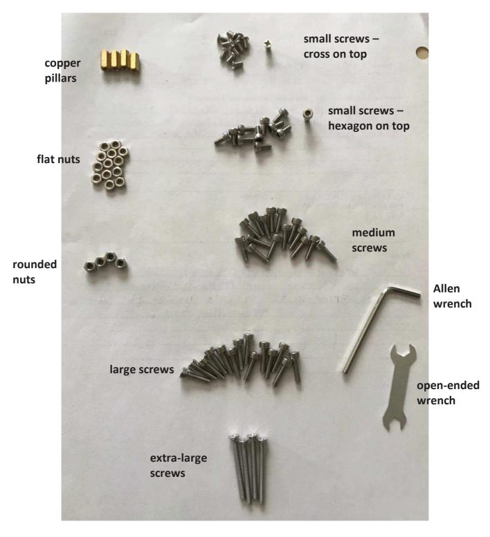
Note: There is not much difference in size between the medium screws and the large screws.
