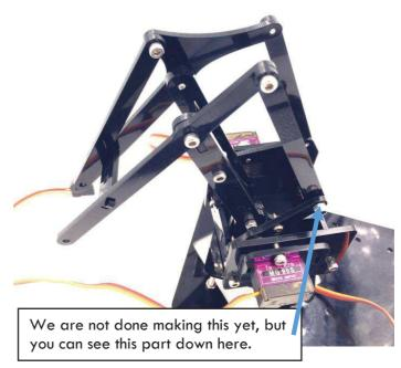
49. Use the small screw to connect the other side of the plastic to the long piece you just installed. Test to make sure your servo can move fully. We want these screws to be pretty loose.
