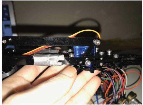
72. Put the robotic arm back on the base. Press down to pop the servo blade into the servo below it.
