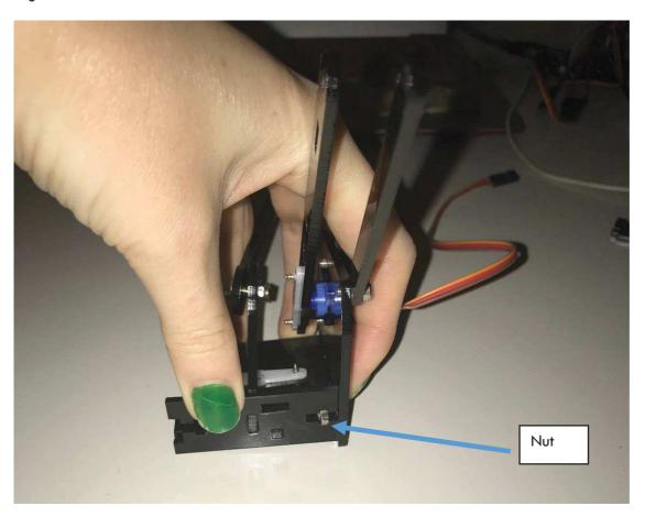
36. Put a screw in the hole at the side. Use the Allen wrench to screw it into the nut.
