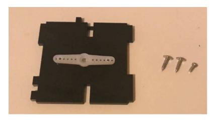
11. Take the white plastic thing off the base servo and attach it to this black piece of plastic. The pointy screws will make the plastic holes bigger. That's ok!
