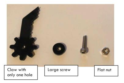
61. On the left side of the Grip servo, put in the screw, then the plastic circle, then the claw, then the flat nut. Screw it just tight enough that the claw doesn't move around.
