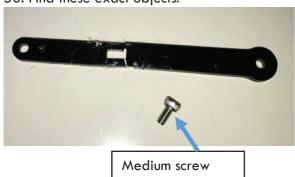
51. Attach this piece of plastic to the bottom hole on the 3-sided piece. The 3-sided piece is on the outside, this new piece is in the middle, and then the screw goes through the main arm on the inside.
