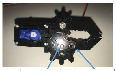
The screw goes in the little hole between the 2 big holes. Line this hole up with the one below it on the grip.
