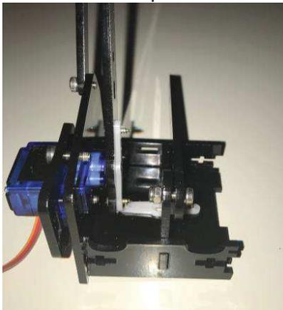
39. Use a screw and nut to connect this like you did before. Use the Allen wrench to tighten the screw.
