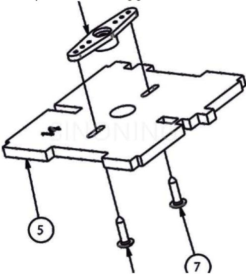
12. Use the very tiny screw to attach this black piece of plastic to your base. Make sure it is facing the right way!
