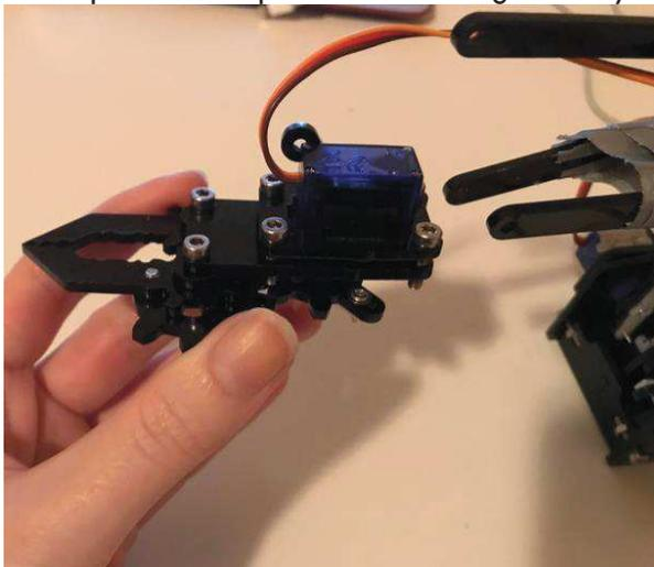
69. Use a medium or large screw to attach the left side. Do not make this very tight.
