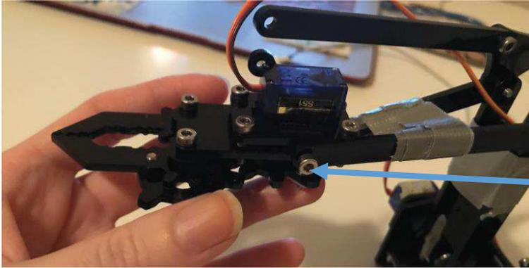
The screw needs to go into a hole in this piece. You may need to loosen other screws to make this work.
