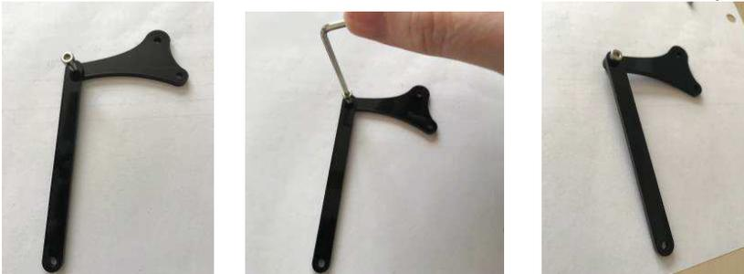
5. Notice that the two pieces of plastic stick together because you put the screw through the big hole first, then the small hole.
