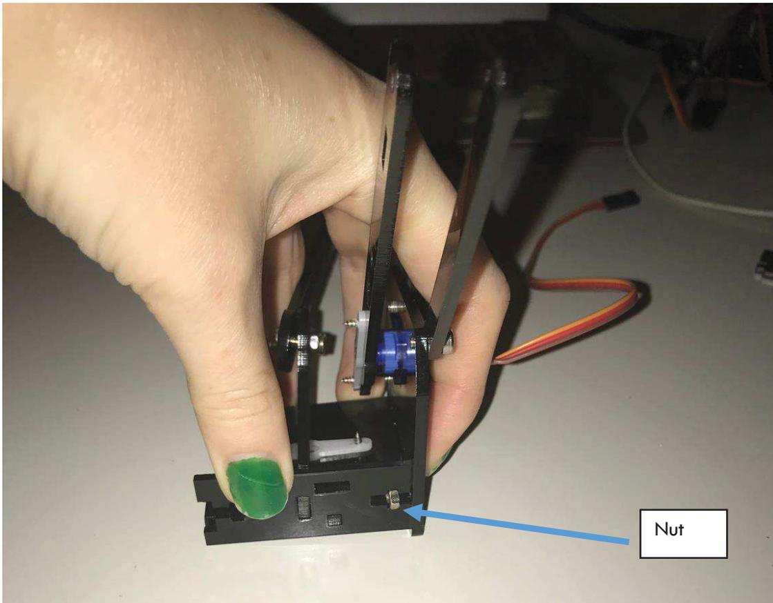
36. Put a screw in the hole at the side. Use the Allen wrench to screw it into the nut.
