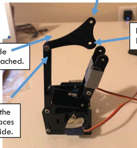
46. Find these exact objects. Flip your robotic arm around. Use the screw to attach the middle of the plastic piece to the other arm on the other side.
