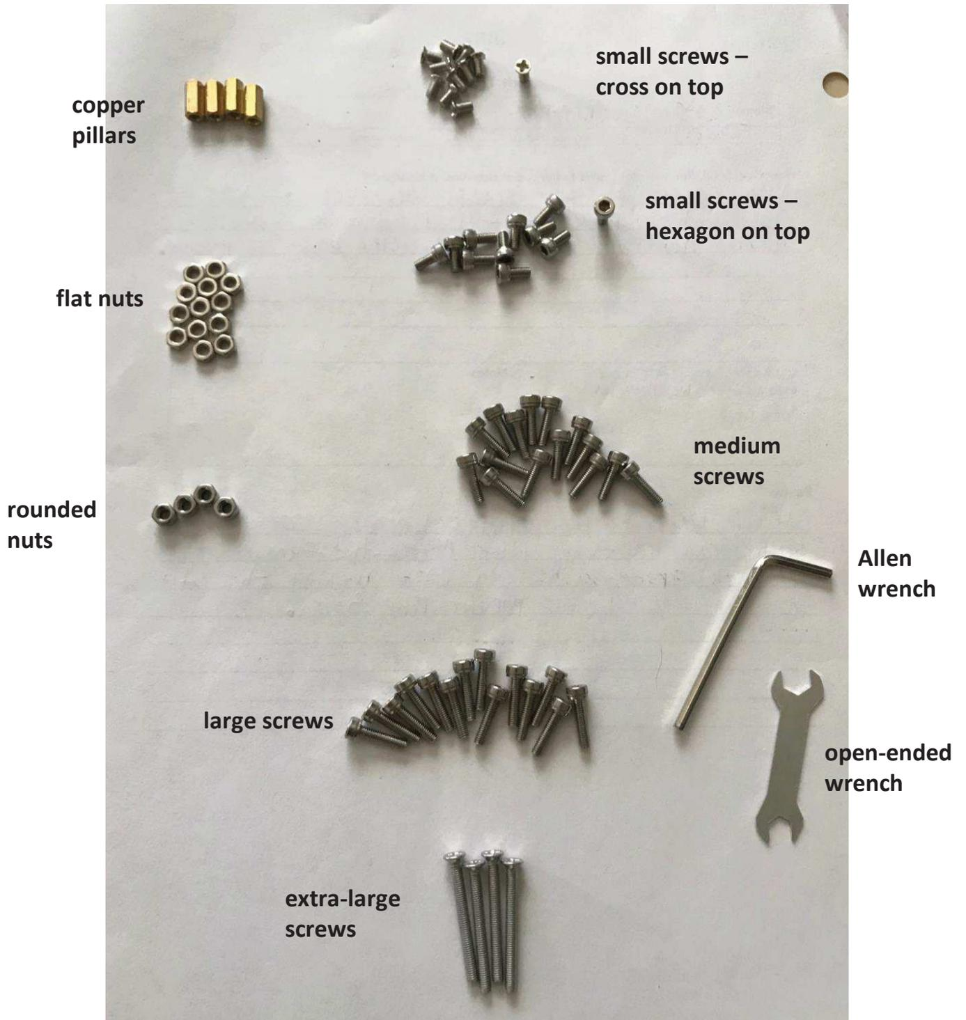
**Note: There is not much difference in size between the medium screws and the large screws.**
