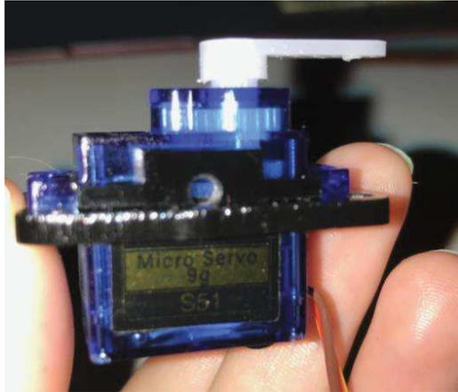
58. Put the large piece on the top. The bigger part should be facing the white blade and the wires. Use the 4 screws to hold it in place. Plug the grip servo back in and check that it still works.
