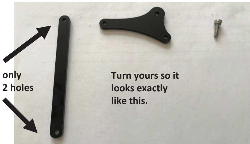
2. Try putting the screw through each hole in the plastic. Notice that on the long piece of plastic, it goes through each hole easily. On the other piece of plastic, it goes through one of the holes easily. It would have to be screwed into the other two holes.
