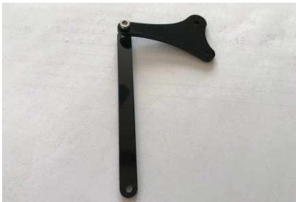
9. Notice that this does not hold the two pieces of plastic together. When you are making your robot arm, if things are not sticking together, it might be because you put a screw through a small hole before a big hole.
